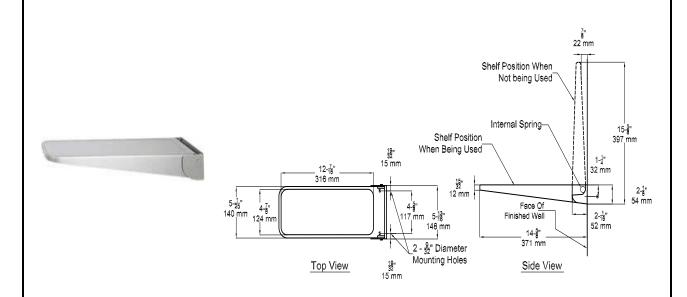
**MATERIALS:** Shelf: 18-8, type 304, No.18 gauge stainless steel. Bracket: 18-8, type 304, No.14 gauge stainless steel.
