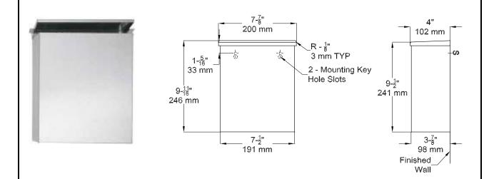
MATERIALS: The unit is fabricated of alloy 18-8 stainless steel, type 304, 22 gauge, No. 4 satin finish.
