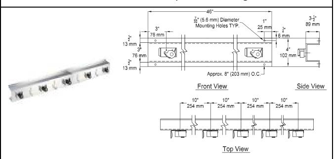
MATERIALS: Rack is fabricated of one piece alloy 18-8 stainless steel, type 304, 20 gauge (.9 mm) with No. 4 satin finish.
