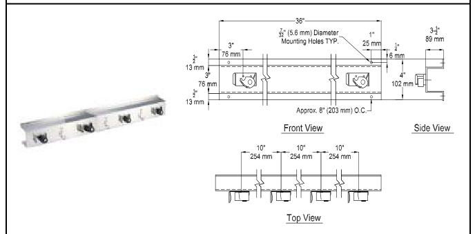
**MATERIALS:** Rack is fabricated of one piece alloy 18-8 stainless steel, type 304, 20 gauge (.9 mm) with No. 4 satin finish.
