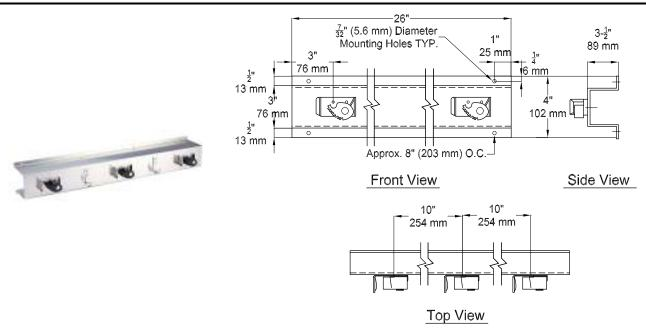
**MATERIALS:** Rack unit is one piece fabricated of alloy 18-8 stainless steel, type 304, 20 gauge (.9 mm) with No. 4 satin finish.
